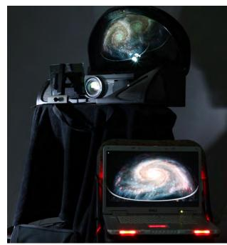
The Discovery Dome utilizes a mirror projection system, called the Newtonian, which delivers sharp, bright images in high definition (1920 x 1080 pixels). It is compatible with a variety of high resolution projectors and can be upgraded when newer projection technology becomes available. We also offer a full range of fisheye solutions using Elumenati projectors.
